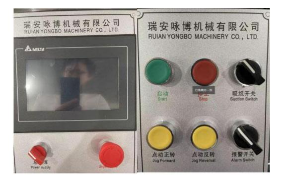
This **Open Cam Single Plate Paper Cup Machine** Control panel with good quality switches, temperature controller and speed converter. All the operation of machine can be finished easily by this panel.
