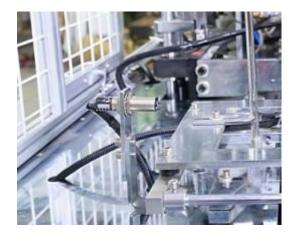
Encoder and the sensor control the machine at the same time, one paper fan match one bottom, no waste.
